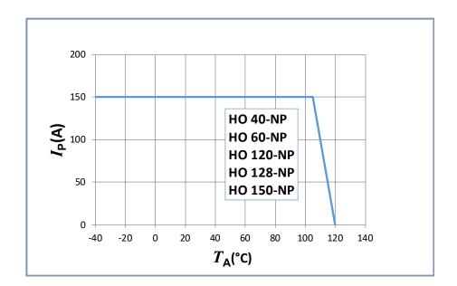
Important Notice: Whatever the usage and/or application, the transducer jumper temperature shall not go above the maximum rating of 120 °C as stated in page 3 of this datasheet.
