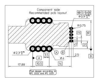
(Layout example with 4 jumpers in parallel)
